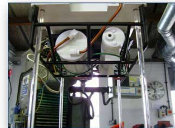
Very detailed parts like internal pressure tanks were manufactured as SLA Rapid Prototype parts
