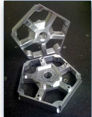
CAD model data generated to enable CNC machining from solid aluminium
