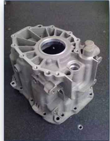
Rapid aluminium casting process Direct from 3D CAD model data
