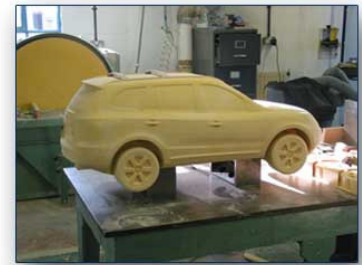
CNC machining used to produce this 4x4 from the manufacturers 3D model data
