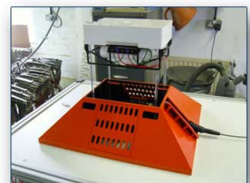
Following assembly of the machined and Rapid Prototype component parts the model was painted to the clients colour scheme
