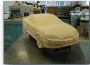
CNC machining from high density modelboard from manufacturers 3D model data
