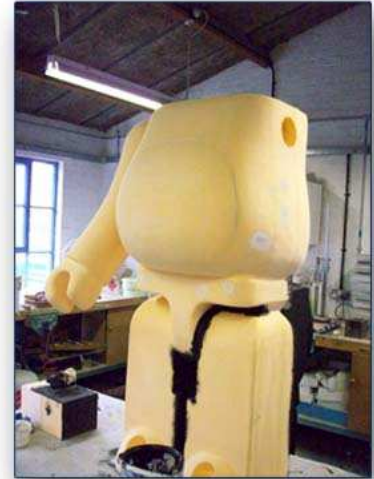
Clients 3D CAD model utilised to enable CNC machining of the foam sections
