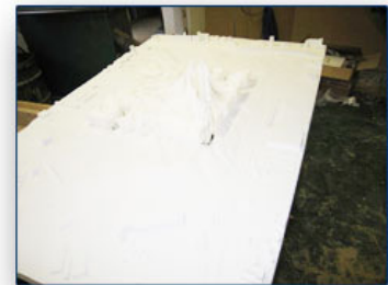
Competition model constructed using CNC machining and rapid prototyping techniques
