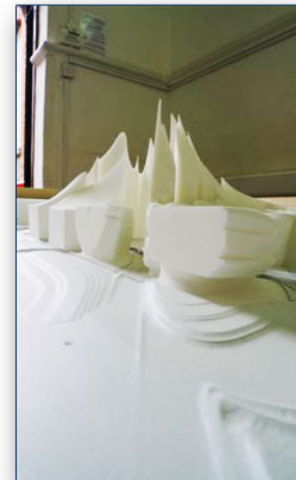
Surrounding landscape created using 3D CNC machining in one piece of high density model board
