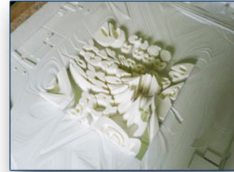
Feature buildings are Rapid prototypes built directly from the client's 3d model data
