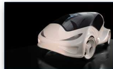
Rapid Prototype and CNC machining processes employed to create these high level models
