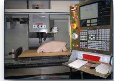
CNC machining of the main body from the clients 3D model data
