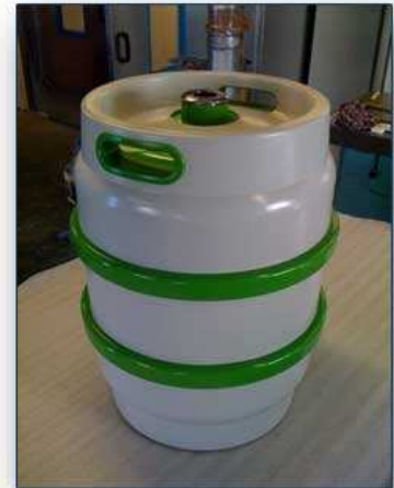
CNC turning used to produce a prototype beer keg exhibition model
