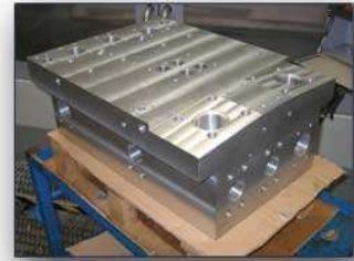
CNC machining of large hydraulic manifold
