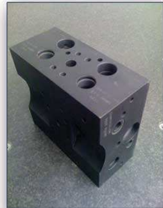
Ancillary manifold CNC machined from 3D model data
