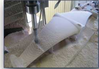
3D CNC machining of the wing section in Ureol
