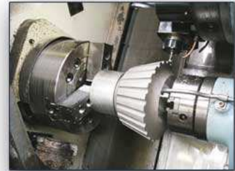
CNC machining of main façade casting
