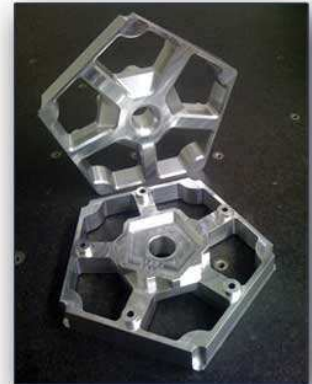
Aluminium CNC machining direct from 3D model
