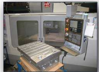
Mainfold CNC machined on our largest Haas VF7
