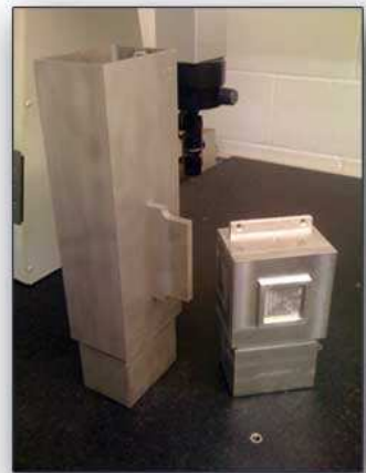
CNC machining of main support casting
